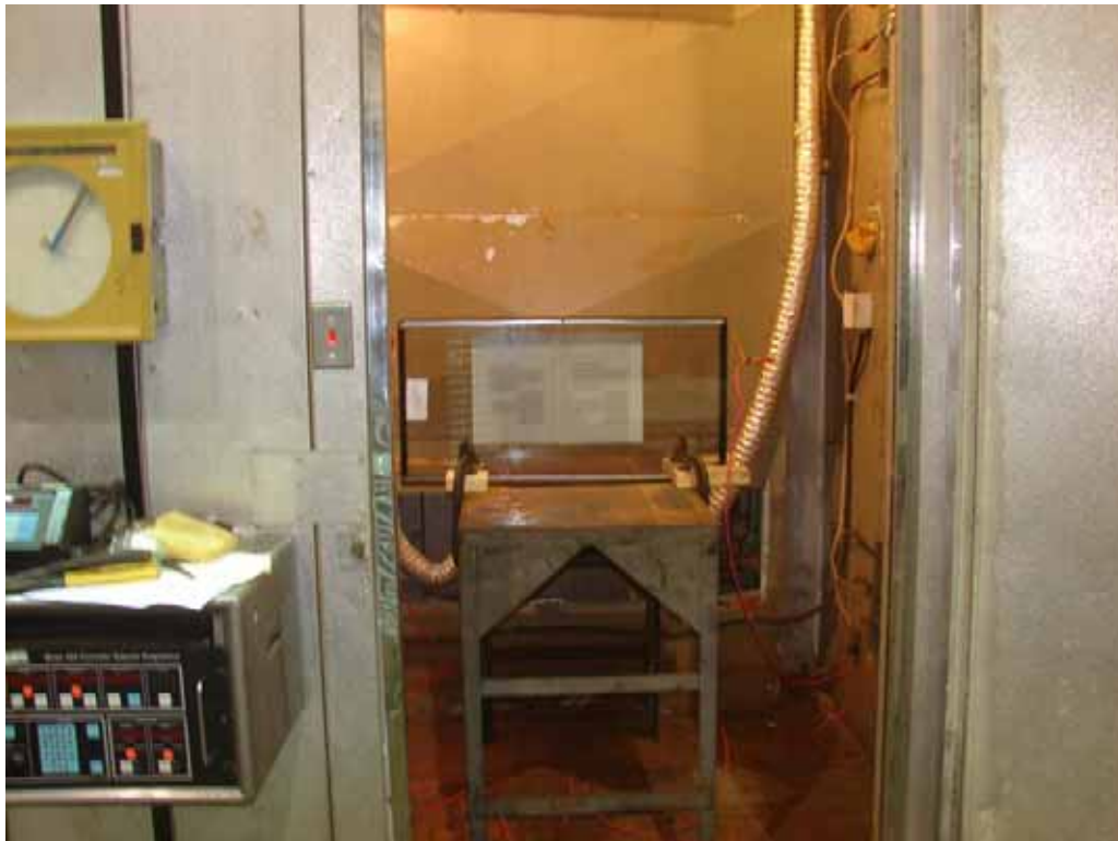
Figure 1. Transparent Armor Windshield in the Environmental Chamber
