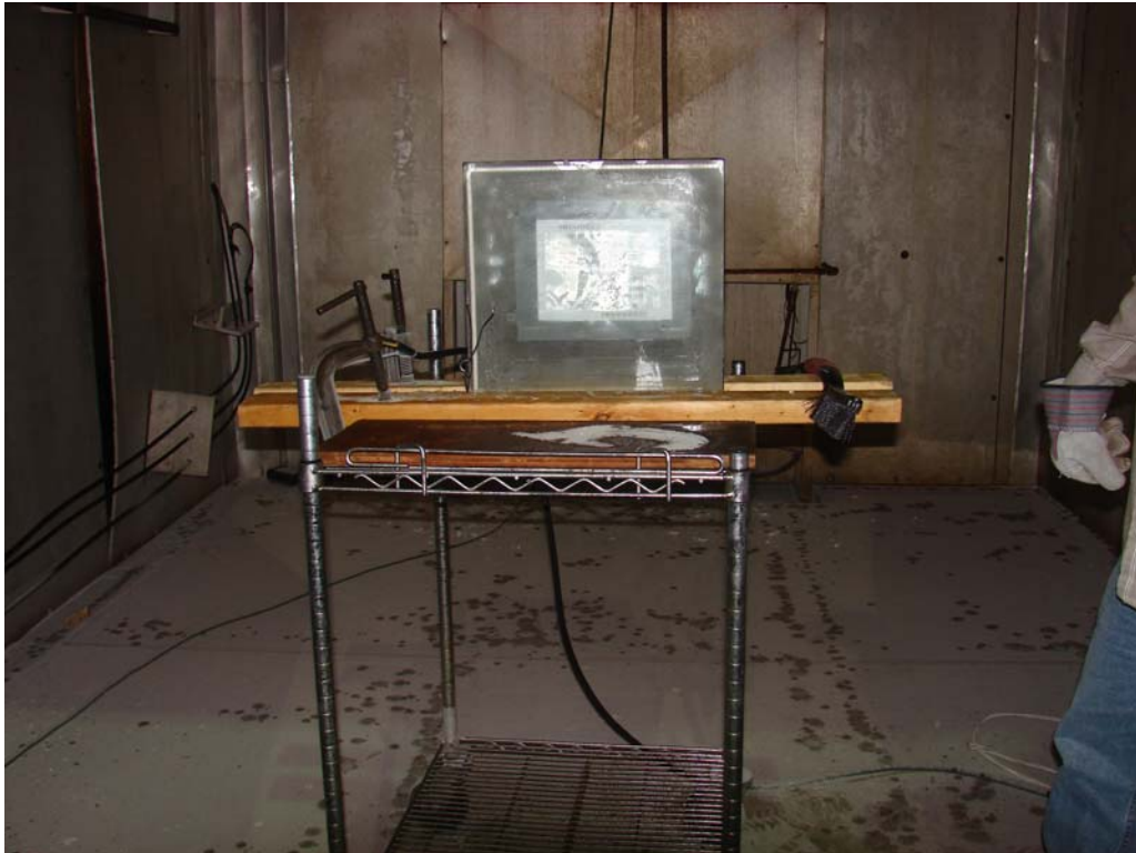
Figure 1. Transparent Armor Windshield in the Environmental Chamber
