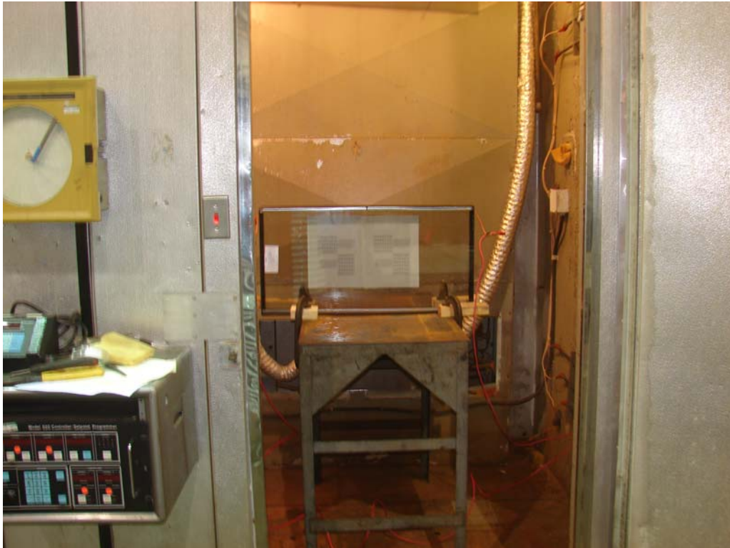
Figure 1. Transparent Armor Windshield in the Environmental Chamber
